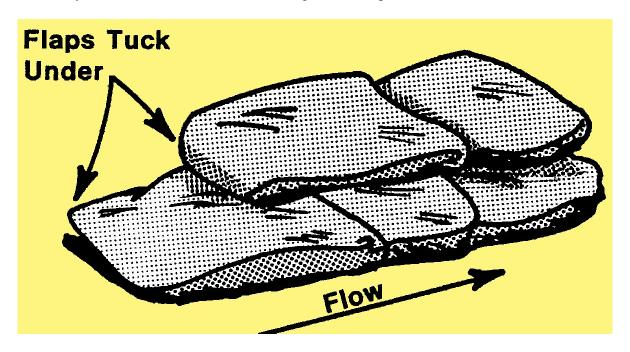
Fold the open end of the unfilled portion of the bag to form a triangle. If tied bags are used, flatten or flare the tied end.
